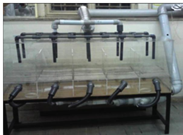
**Figure 1.** Inhalation Chamber Used for Whole-Body Inhalation Exposure to Carbon Black PM10
