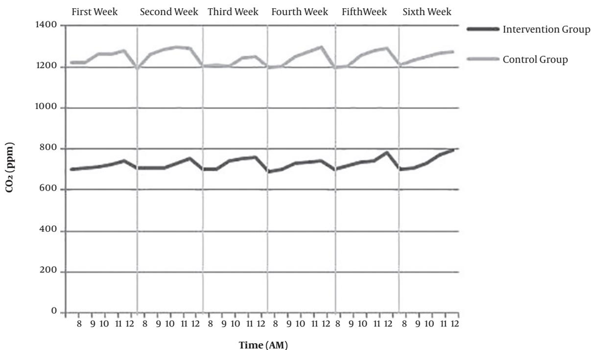
Figure 1. Indoor CO<sub>2</sub> concentration during 6 weeks in the intervention and control groups
