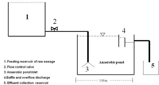
**Figure 1.** Schematic diagram of pilot anaerobic stabilization pond system
