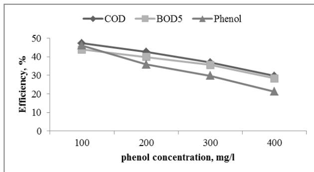
**Figure 2.** Efficiency of anaerobic pond of Kermanshah oil refinery in different concentrations of phenol
